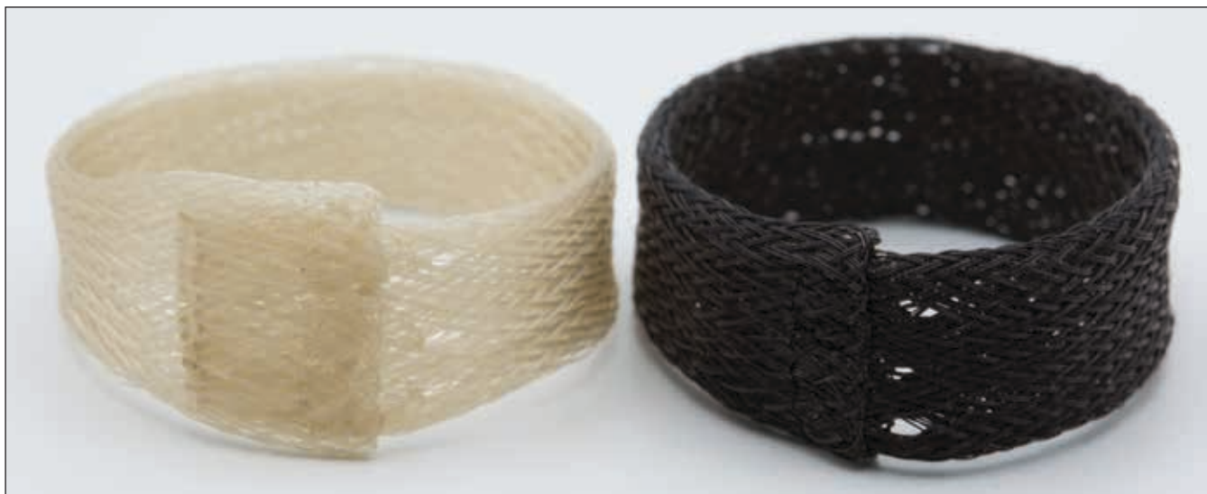
In the medical industry, PVD coatings can provide radiopaque layers, as with this woven polyetheretherketone (PEEK) after tantalum coating.
