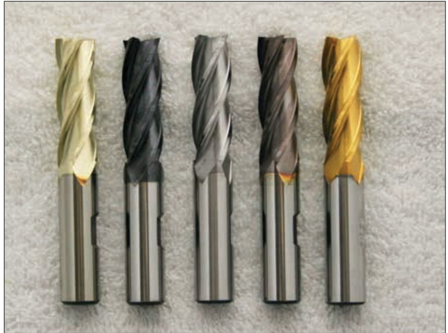
In the tool coating arena, the main purpose of the coating is to control the friction and wear of a specific surface on a cutting or forming tool.
